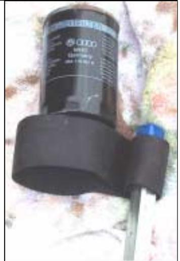
Figure 2. Oil Filter w/ wrench
