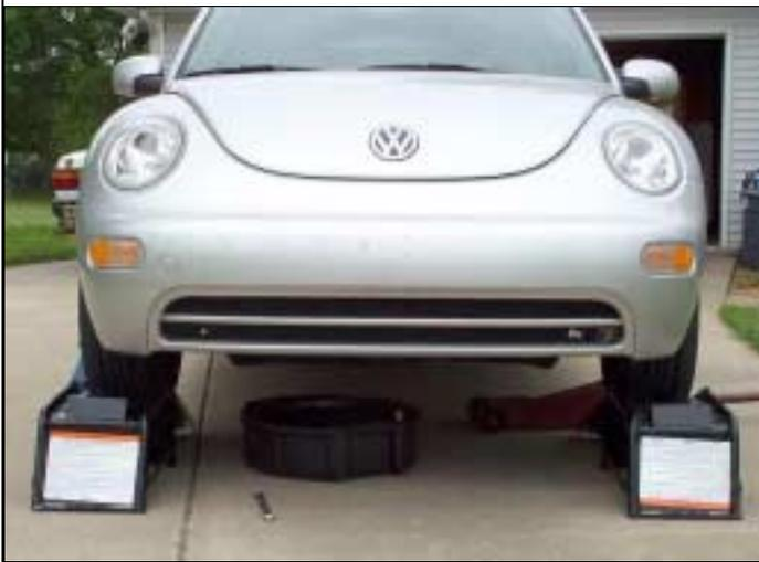
Figure 1. Using a floor jack to place NB on ramp.
